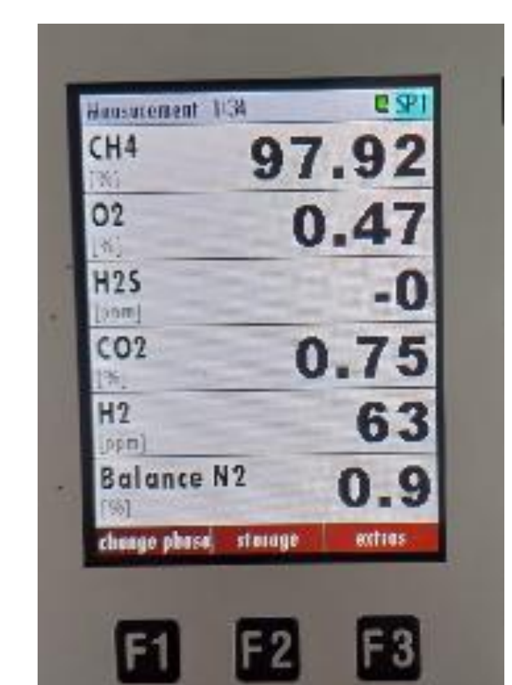
Figure 3. Gas analysis system for real-time monitoring of biomethane composition connected to DSS (KER4)
