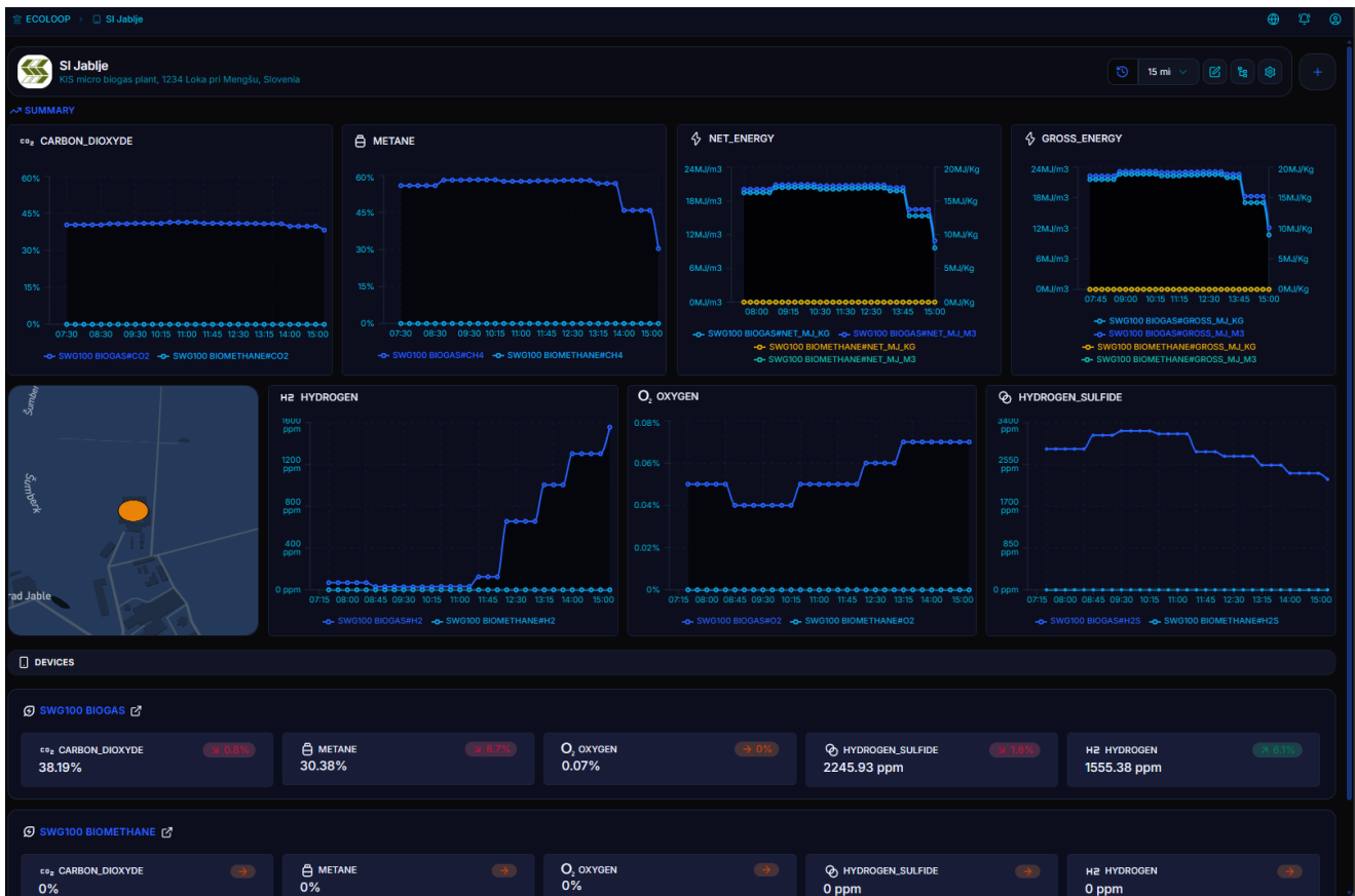
Figure 24: KIS dashboard where both biogas and biomethane data can be displayed
