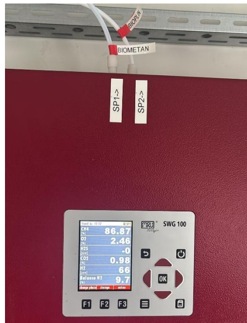
Figure 23 SWG1000 analyzer that analyzes both biogas and biomehtane
